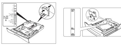
For the FAX-L390 model, be sure to properly attach the stopper of the paper size rear guide for the correct paper size by inserting the tabs into the matching slots on the paper cassette.
